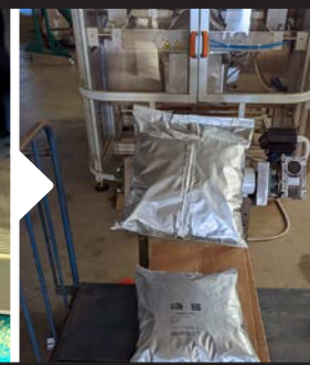
PROTECTIVE GAS INJECTION, HEAT SEALING & BAG CUTTING
